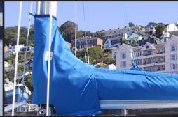
Adjustable batten pockets sewn close to top so that water does not accumulate in the cover when sail is away in the cover
