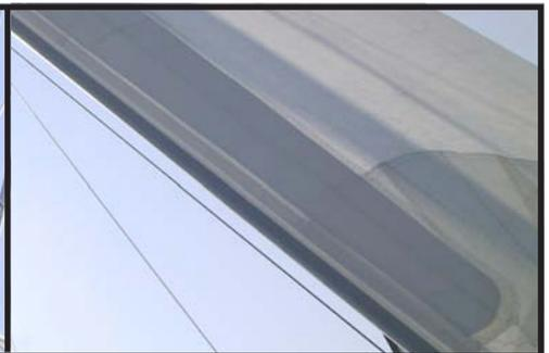
Option of foam padded luff to remove excess camber when the sail is part furled.
